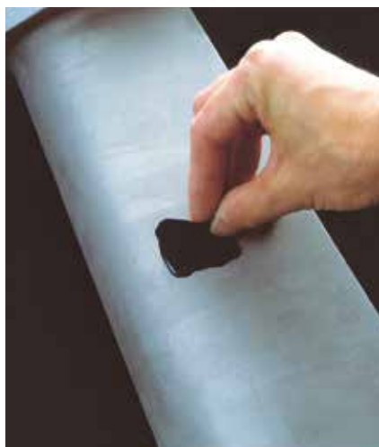
An operator peels off the cured replica
